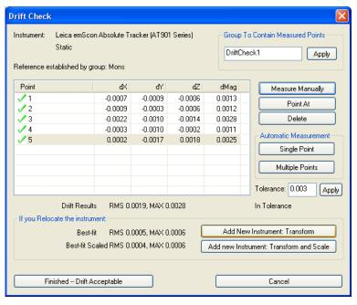
Two new buttons: Add New Instrument: Transform and Add new Instrument: Transform and Scale will conveniently add another instrument, activate its interface, and place you into a completed *Measure Nominals* dialog, allowing you to apply a best fit or best fit with varying scale without measuring any additional points.
