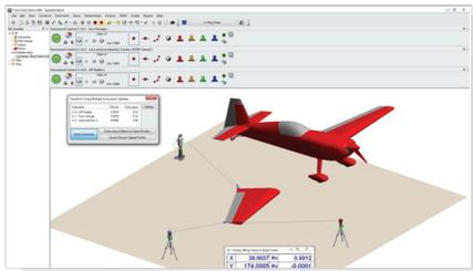
SA can simultaneously communicate with virtually any number and type of portable metrology instruments. This includes laser trackers, arms, laser radars, scanners, projectors, theodolites, total stations, and photogrammetric devices—all featuring a common interface for each instrument class.
