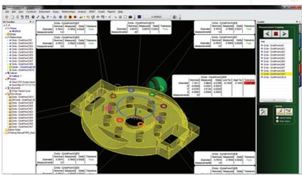
Define design-based inspection routines from a CAD model or primitive geometry.
