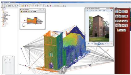
Combine laser scanner interfaces with advanced tools for feature fitting and automatic sphere extraction. Automatically extract features from scan data for easy comparison to CAD or analysis with GD&T.
