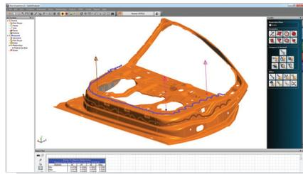
Align to a known coordinate system using a variety of techniques, from 3-2-1 and best fits to interactive fitting such as Quick-Align and classic surface fits. Relationship Fitting allows for simultaneous feature-based fitting to organic surfaces in addition to traditional iterative fitting.
