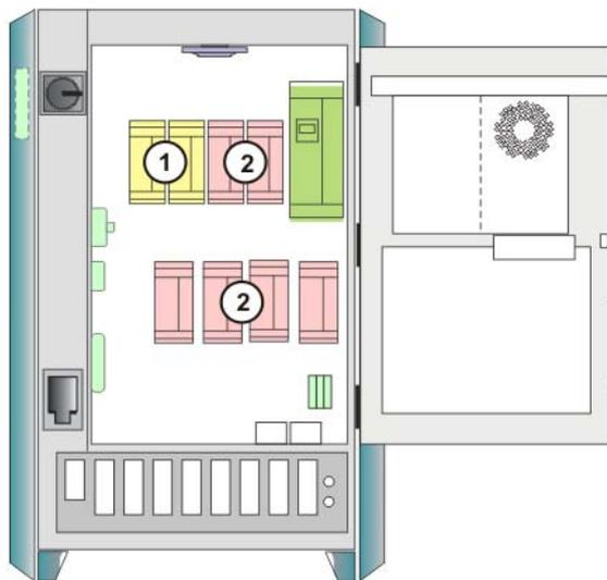
**Fig. 3-1: KSDs in the robot controller**
