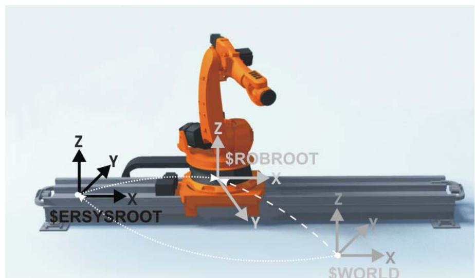
Fig. 5-2: ROBROOT kinematic system – linear unit
