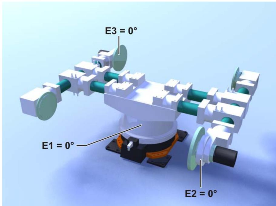
**Fig. 6-1: Example of mechanical zero position**
