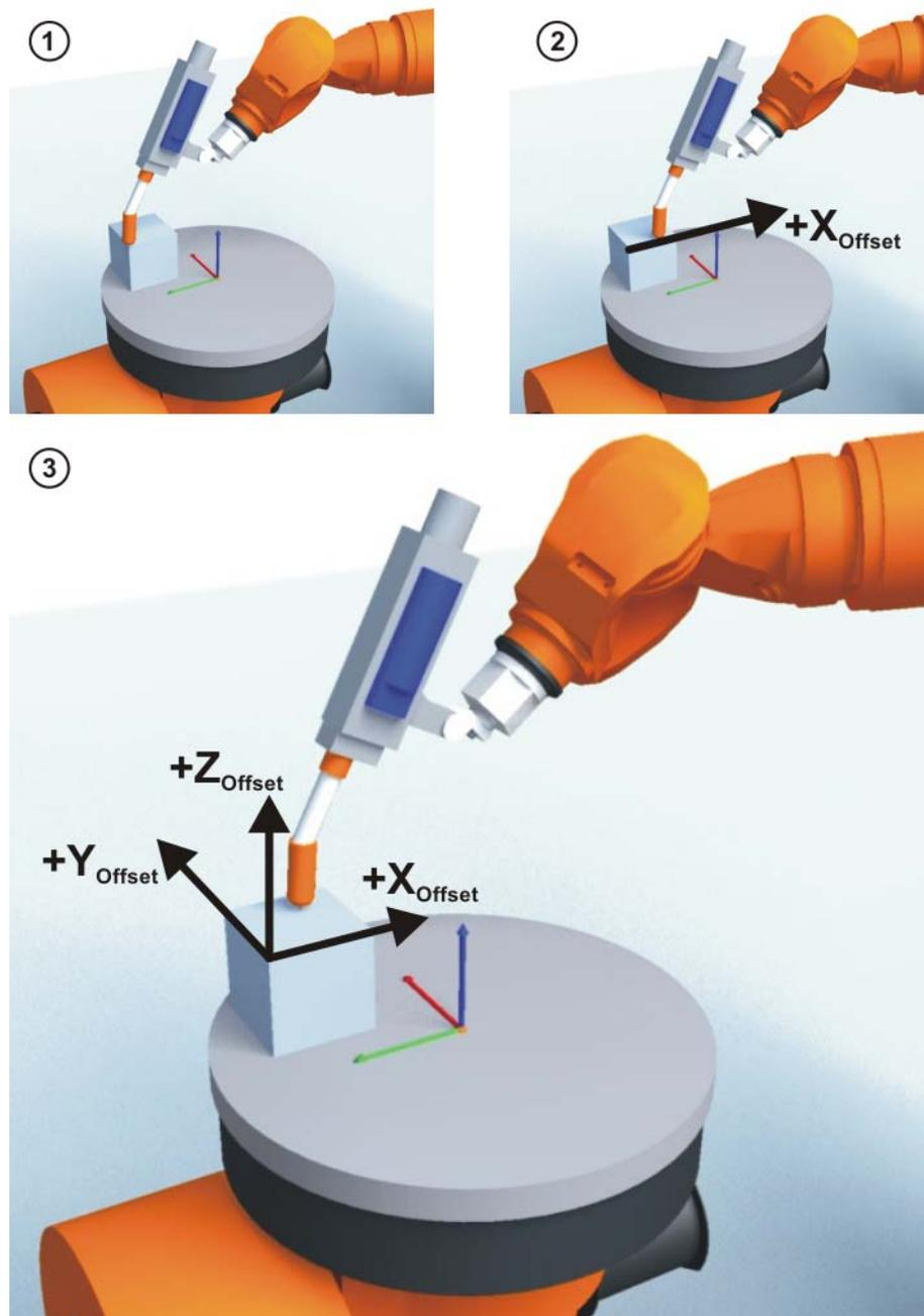
Fig. 6-8: Offset base calibration principle
