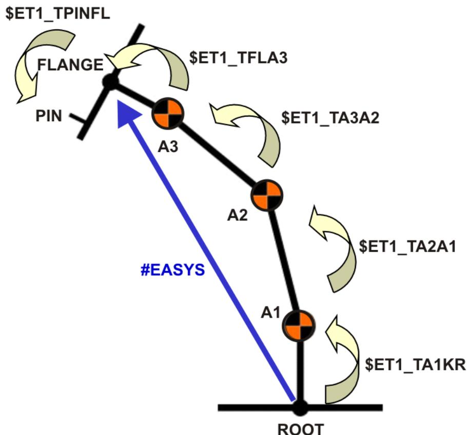
Fig. 7-1: Transformation chain of a BASE kinematic system
