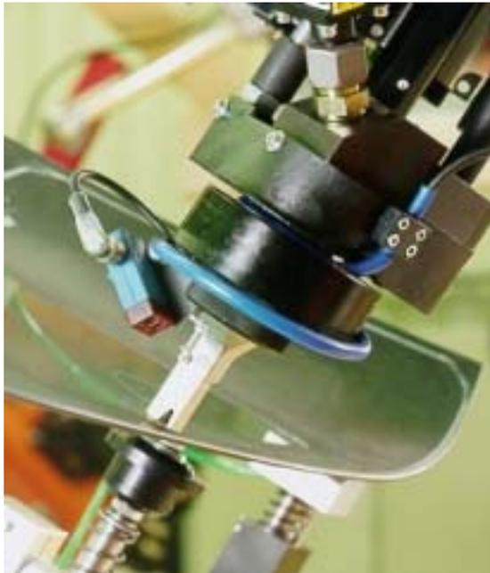
Fig. 2-4: External adhesive nozzle
