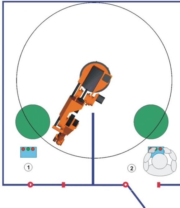
**Fig. 2-7: Diagram: system with synchronous and asynchronous external axes**
