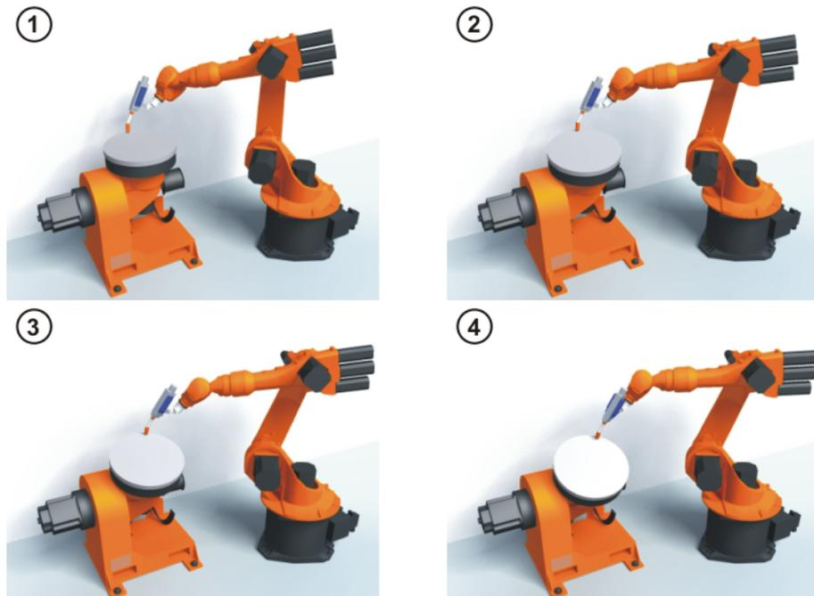
Fig. 6-7: Root point calibration principle
