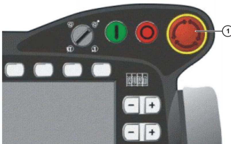
Fig. 4-4: EMERGENCY STOP button on the KCP
