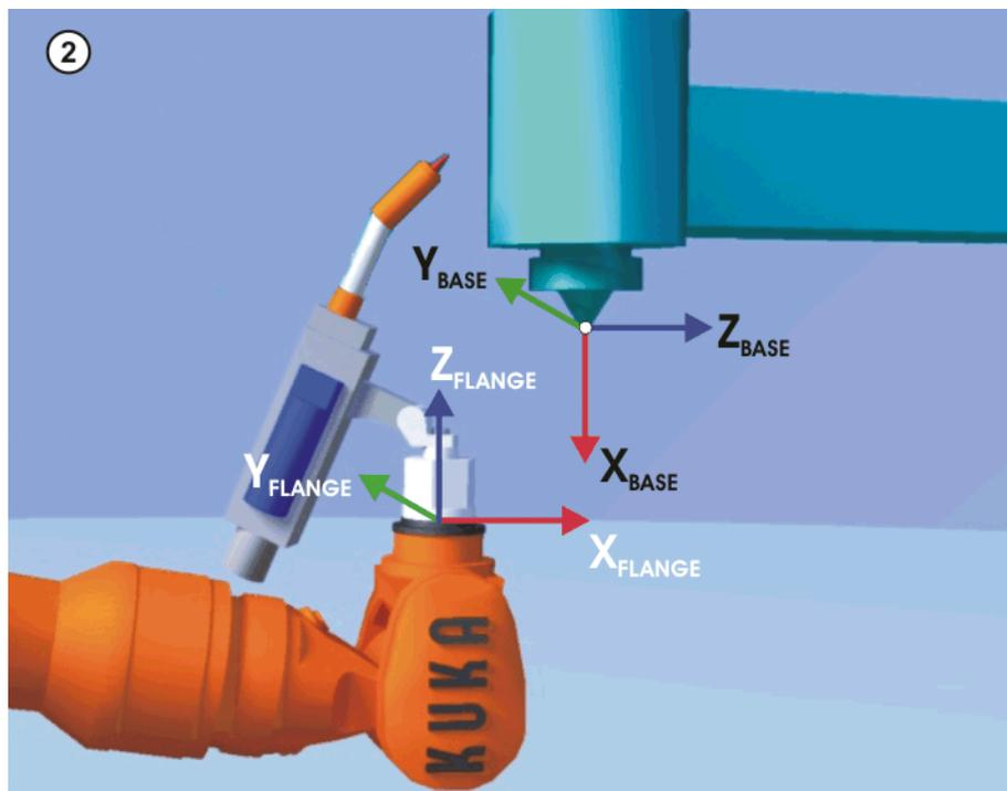
Fig. 6-10: Aligning the coordinate systems parallel to one another
