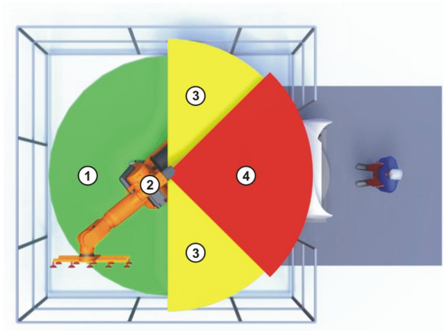
Fig. 4-3: Example of axis range A1
