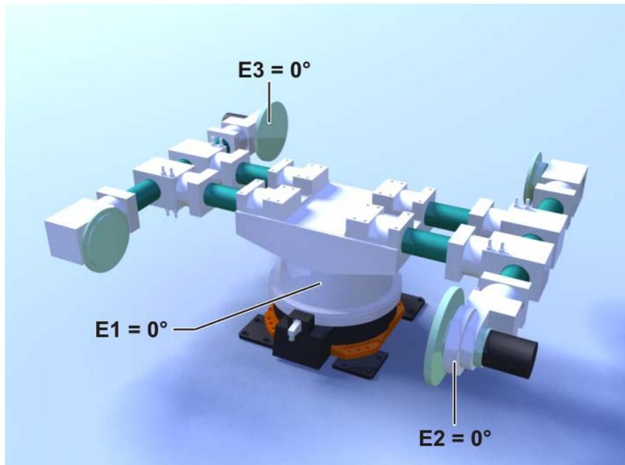
**Fig. 6-1: Example of mechanical zero position**
