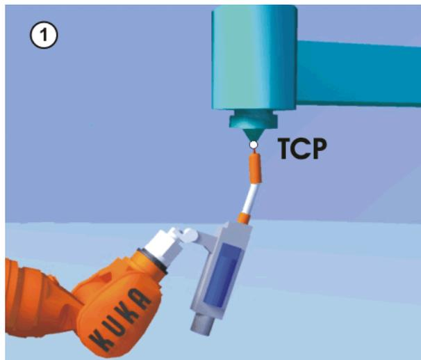
Fig. 6-9: Moving to the external TCP
