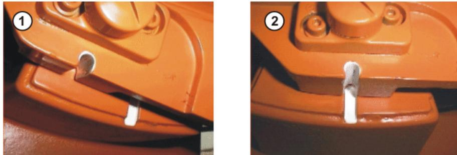
Fig. 6-4: Moving an axis to the pre-mastering position
