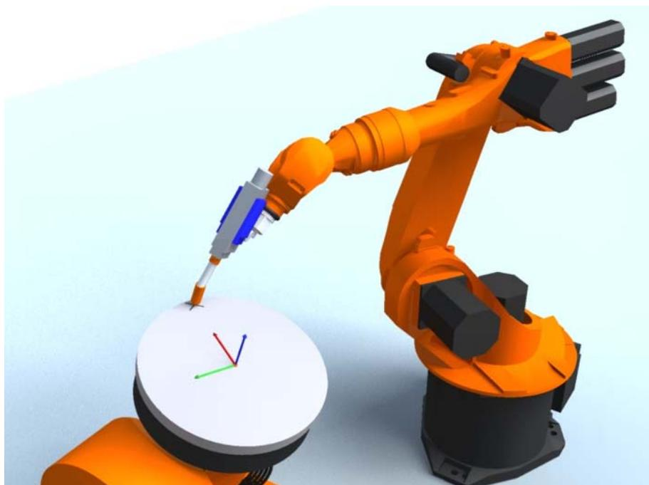
**Fig. 6-6: Mark on DKP 400 for root point calibration**
