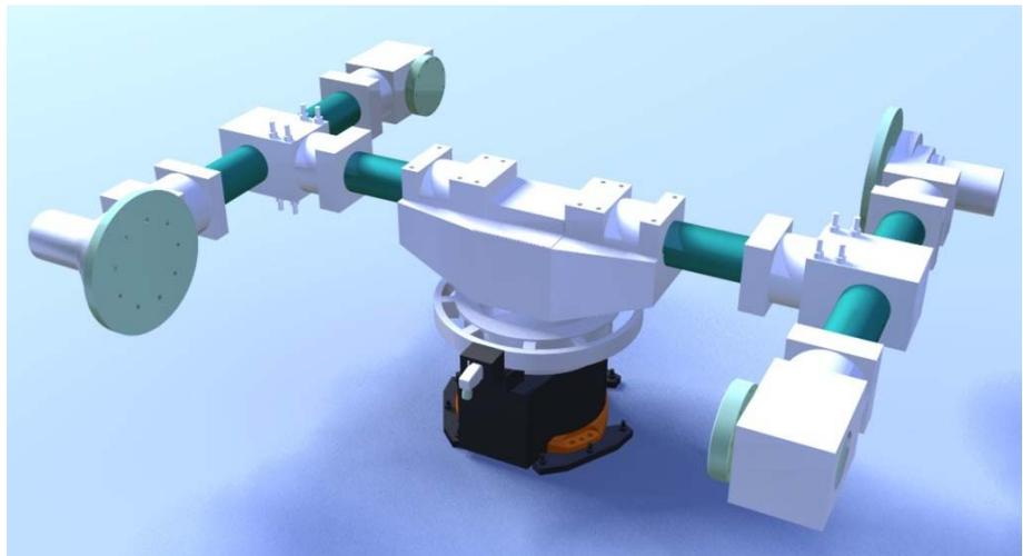
Fig. 2-3: Three-axis positioner
