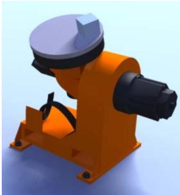
Fig. 2-2: Two-axis positioner
