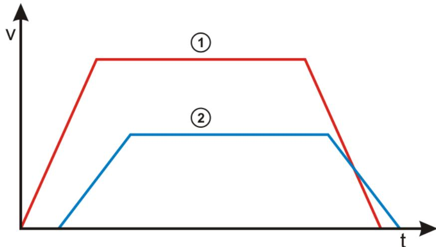
**Fig. 2-6: Asynchronous robot and external axis motion**
