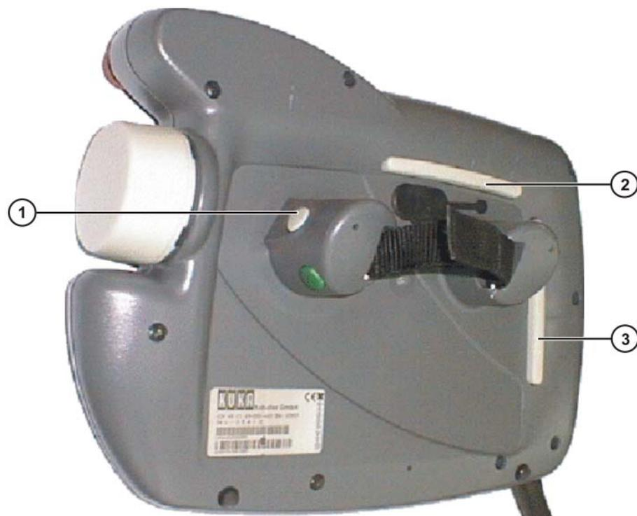
**Fig. 4-5: Enabling switches on the KCP**
