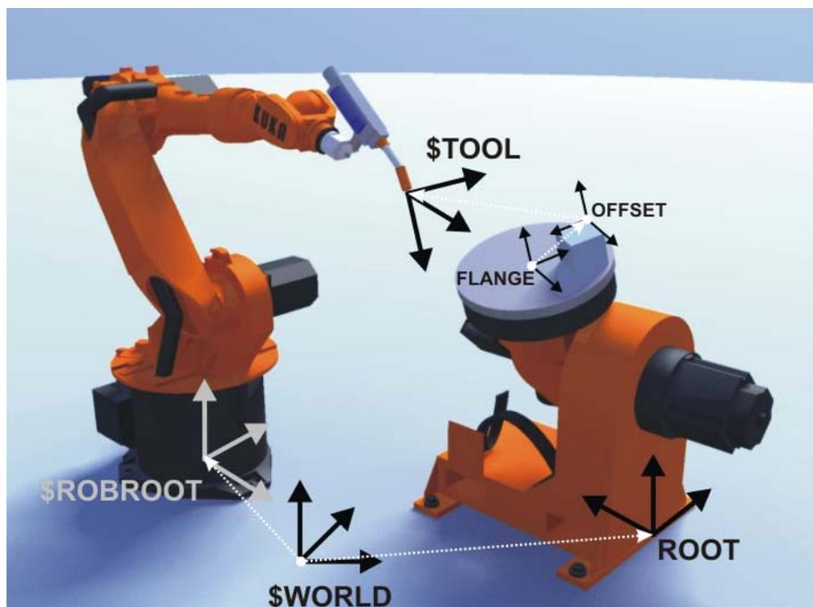
Fig. 5-1: Kinematic chain with DKP 400
