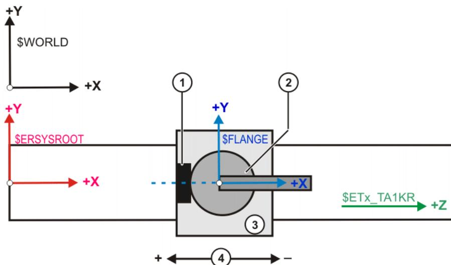
Fig. 10-4: Transformation for linear unit – top view
