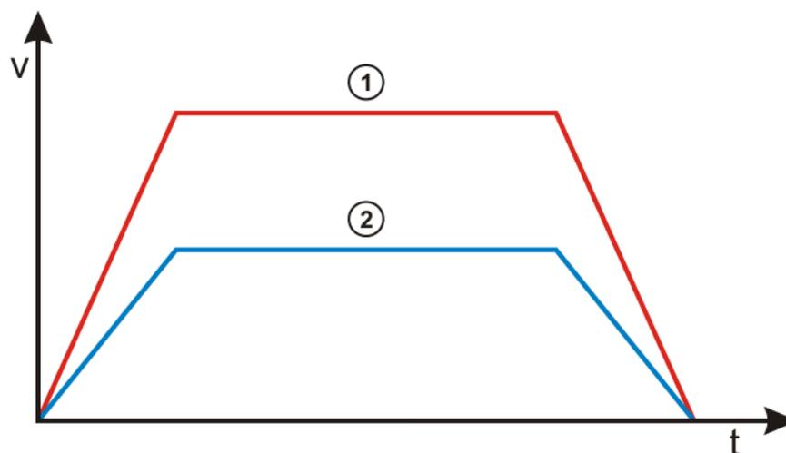
Fig. 2-5: Synchronous robot and external axis motion
