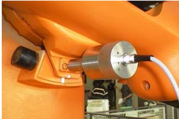
Fig. 6-2: EMT – electronic measuring tool
