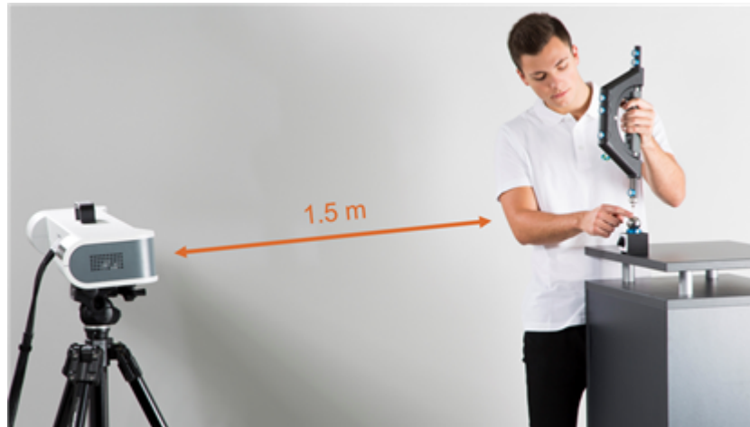
Figure 161: Recommended distance between camera system and calibration sphere
