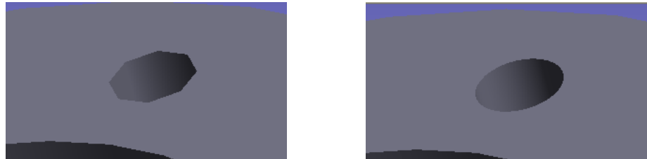
Figure 5-21. Max trimmed edge angle: 65 (left) and 15 (right).
