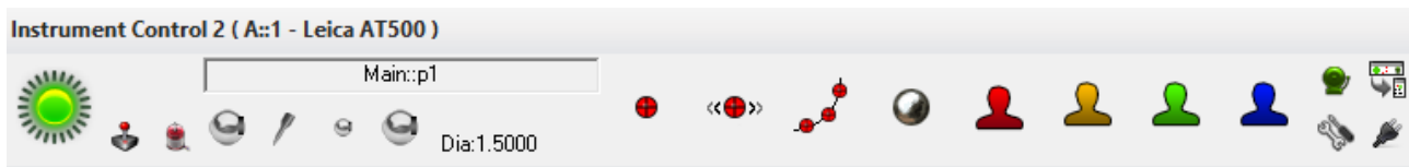
Figure 3-78. Instrument Control Toolbar is a simplified tracker interface to expand graphic space.
