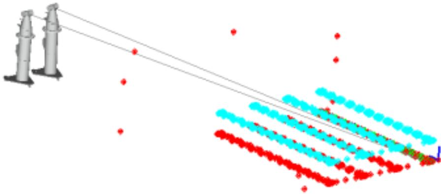
**Figure 15: Test setup of the two laser trackers, measurement points, and machine bed coordinate system frame.**
