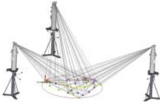
**Figure 12: Three-tracker trilateration network**
