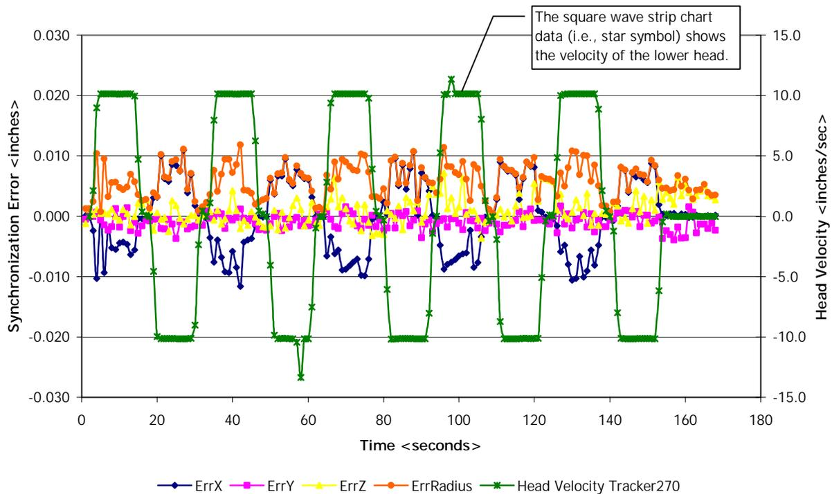
**Figure 17: Synchronization Error between the Laser Tracking Interferometers**
