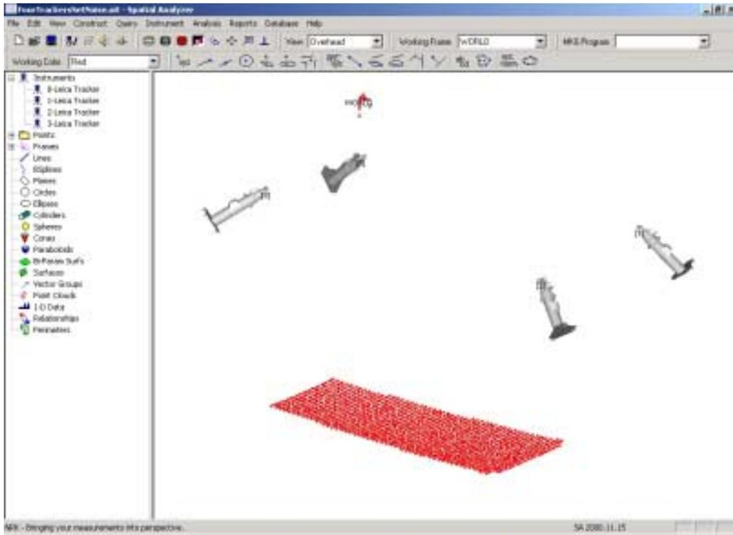
**Figure 1: 4 Laser tracker Trilateration using simulated test data.**
