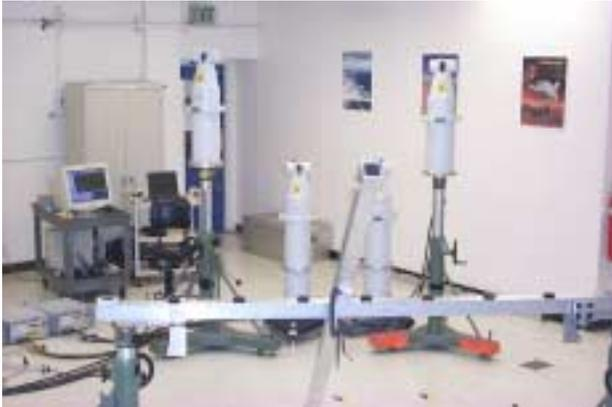
**Figure 8: 4 Laser Tracker Test Setup**
