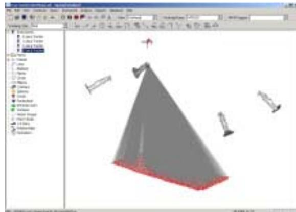
**Figure 3: Trilateration setup, showing the measurements from instrument number 1 of 4.**
