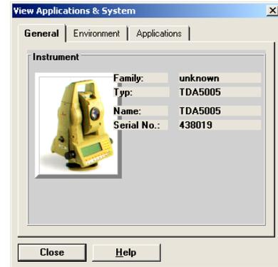
If the Applications tab shows that the NRK\_TS application is already on the instrument. You should be ready to use the instrument with SpatialAnalyzer by restarting the instrument and running the application. If you need to either change or reload the NRK\_TS application please follow the steps in the 'Deleting a prior version of NRK\_TS' section before uploading a new copy.
